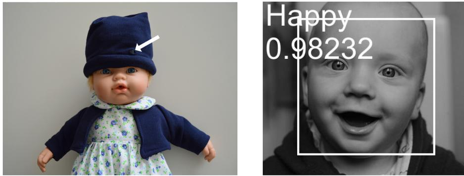
**Figure 24.** Smart doll with emotion recognition. Left: The camera was in the head, connected through a flex cable to the board and battery inside the body. Right: emotion recognition.
