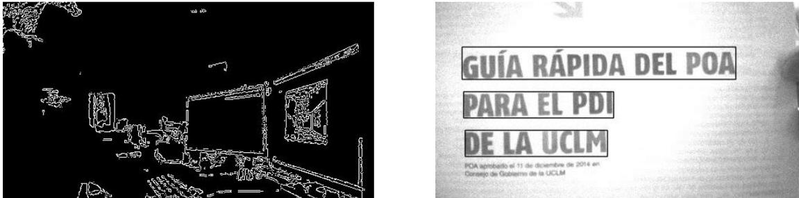
**Figure 14.** Libccv examples running in EoT. Left: Canny edge detection. Right: text detection in images.
