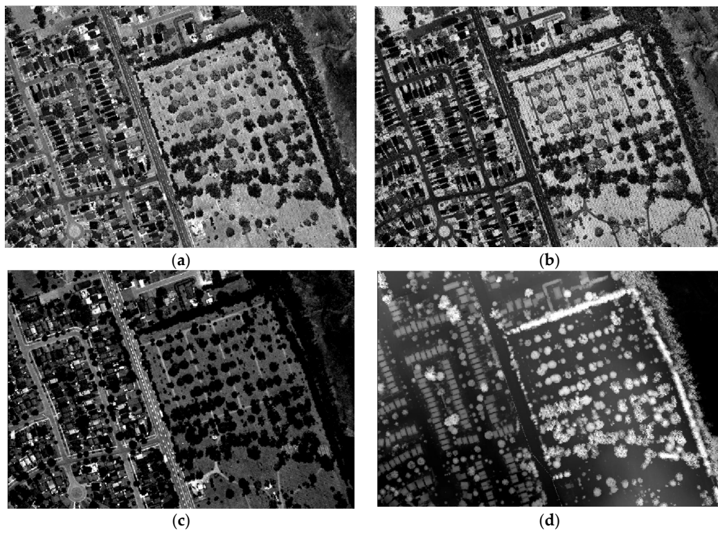
Figure 6. LiDAR raster images: (a) C1 intensity; (b) C2 intensity; (c) C3 intensity; (d) DSM.
