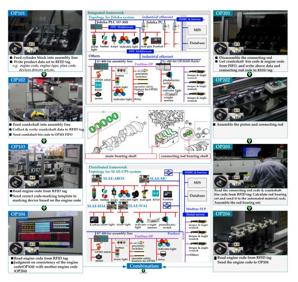
Figure 7. Piston rod assembly region in the engine assembly line.
