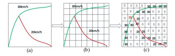
**Figure 3.** Traffic speed representation in a small-scale transportation network: (a) two links with different speeds in a transportation network; (b) the network is divided into several grids (the size of each grid is approximately  $10 \text{ m} \times 10 \text{ m}$ ); (c) the speed of each link is mapped to each grid.
