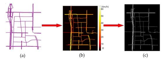
**Figure 2.** Grid-based transportation network segmentation process: (**a**) A transportation network without traffic information; (**b**) the speed of each link is mapped and colored in the network; (**c**) the speed of each link is normalized and greyed in the network.
