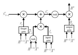
Figure 6. LSTM NN architecture.
