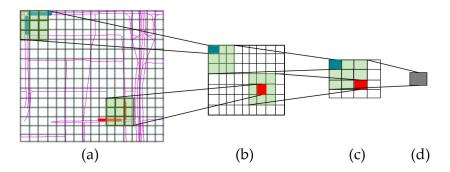
**Figure 4.** Convolutions for capturing near and far dependencies: (**a**) the original transportation network; (**b**) the transformed network with the first convolution; (**c**) the transformed network with the second convolution; (**d**) the transformed network with the third convolution.
