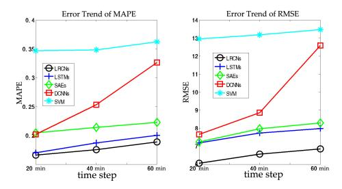
Figure 11. Prediction errors for the prediction horizons (20, 40, and 60) min in terms of MAPE and RMSE.
