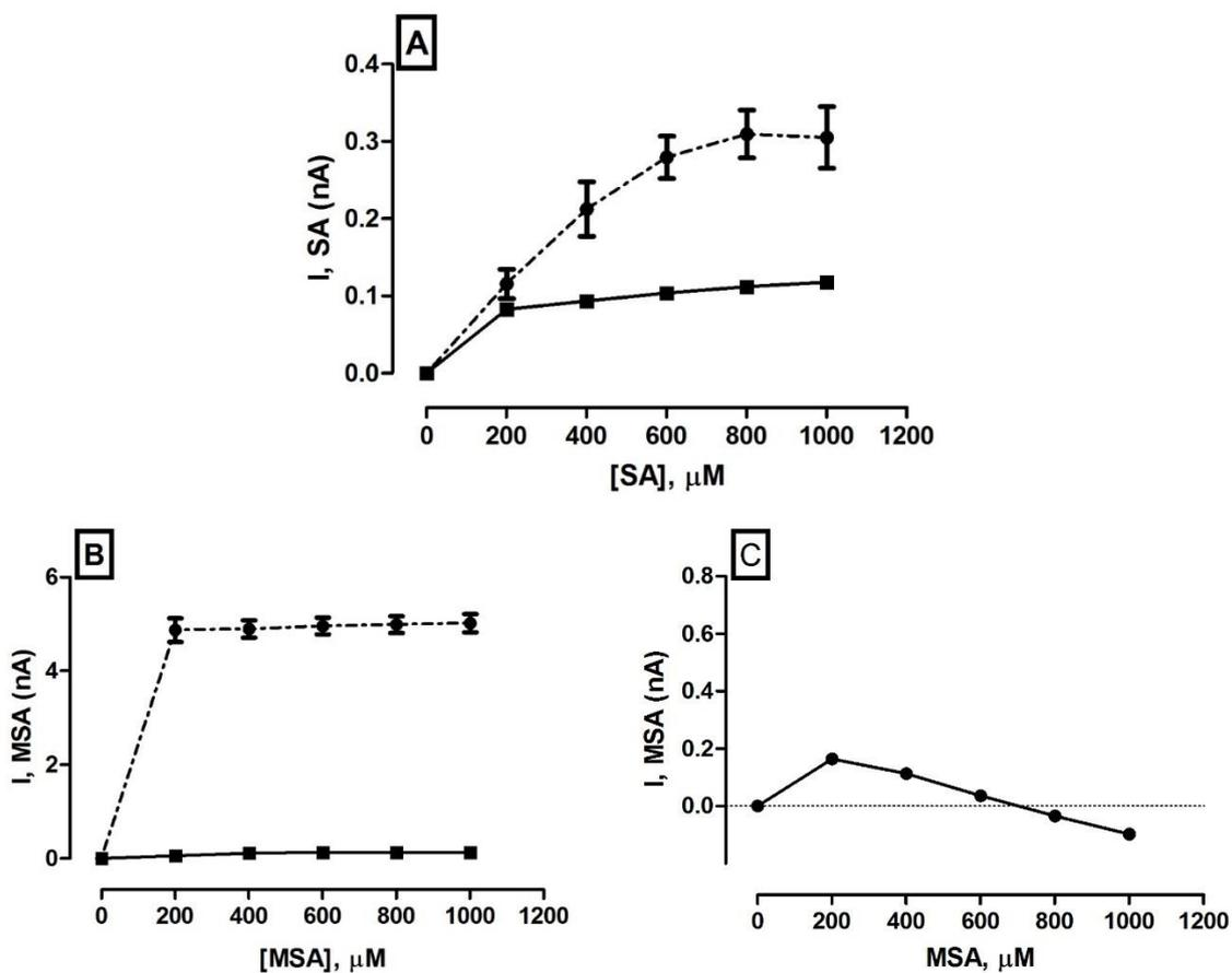
**Figure S6.** Current concentration profiles for (A) 0–1000  $\mu\text{M}$  SA calibration and (B) 0–1000  $\mu\text{M}$  MSA calibrations on unmodified bare Pt electrodes (dashed lines,  $n = 8$ ) and H<sub>2</sub>O<sub>2</sub> blank electrodes (solid lines,  $n = 8$ ). (C) Effect of 0–10 mM H<sub>2</sub>O<sub>2</sub> calibration on MSA rejection characteristics of H<sub>2</sub>O<sub>2</sub> blank electrodes ( $n = 12$ ). All concentration profile data is presented as mean  $\pm$  SEM.
