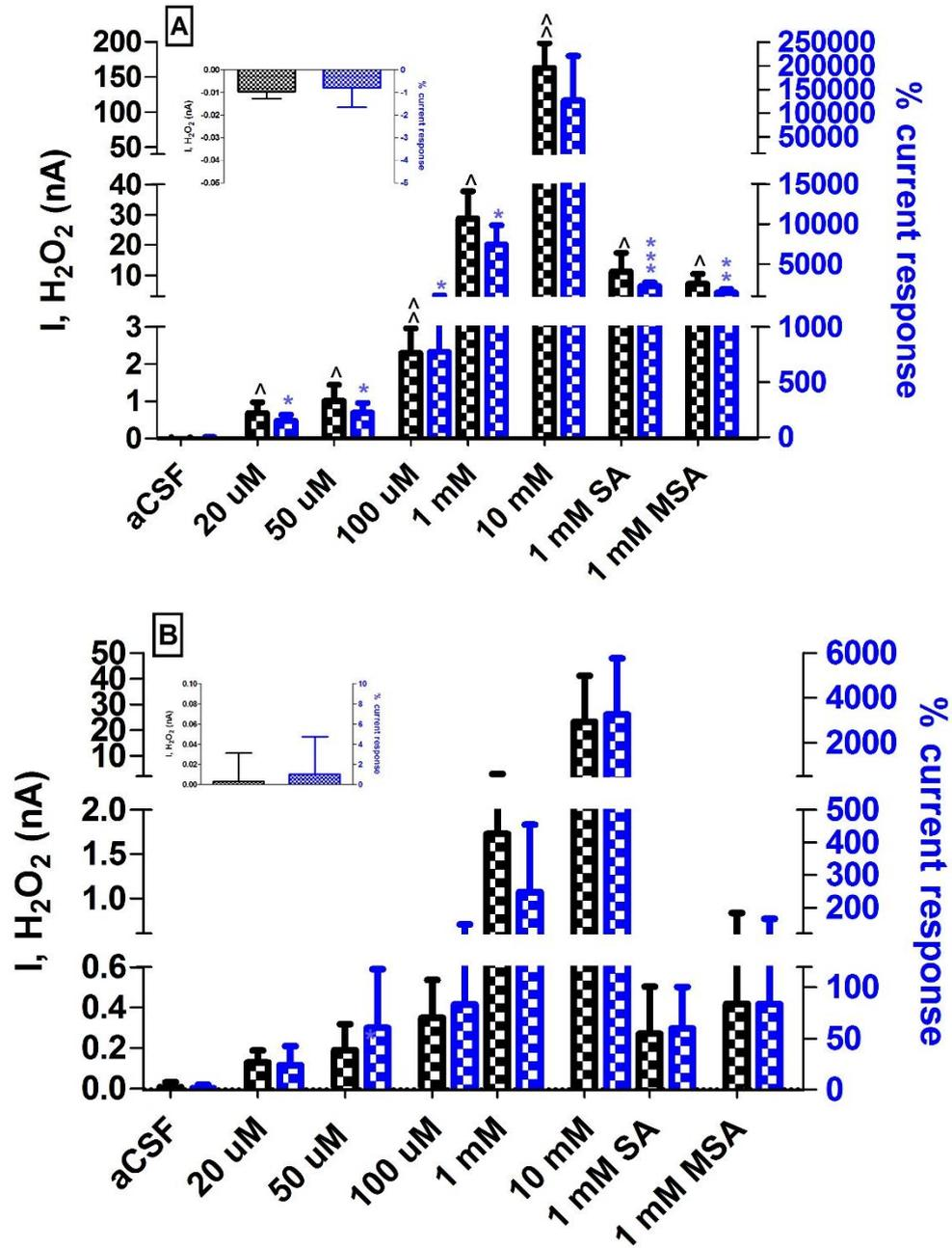
**Figure S5.** Dose effect of infusion of 0–10 mM H<sub>2</sub>O<sub>2</sub>/ aCSF ( $n = 5$ ), 1 mM SA ( $n = 3$ ) and MSA ( $n = 3$ ) on (A) H<sub>2</sub>O<sub>2</sub> blank electrode current and (B) H<sub>2</sub>O<sub>2</sub> catalase electrode current. Current (left y-axis) and % current response (right y-axis) data represented as mean  $\pm$  SEM. ^ and \* denote level of significance for currents and % currents respectively.
