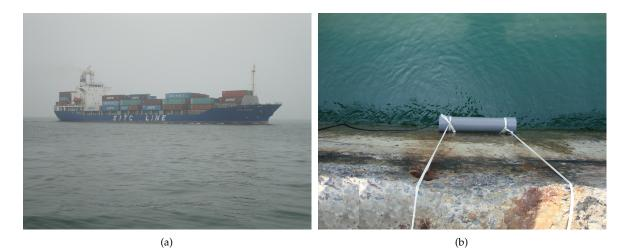
**Figure 2.** The detection experiment on a shallow sea. (**a**) the surface ship as the target; (**b**) the magnetic field sensor above the sea surface.
