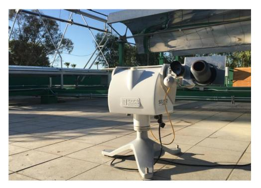
Figure 9. Experimental setup, SOLYS 2 and on its surface the solar position sensor.
