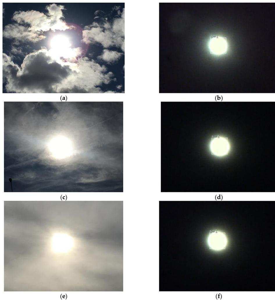
**Figure 7.** Cloudy real images and images viewed through the vision sensor. (a) Real view of the Sun partially cloudy; (b) Sensor view of the Sun partially cloudy; (c) Real view of the Sun nebulous cloudy; (d) Sensor view of the Sun nebulous cloudy; (e) Real view of the Sun cloudy; (f) Sensor view of the Sun cloudy.
