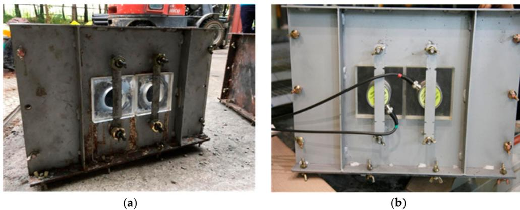
**Figure 2.** Preparation of the steel mold for surface wave velocity measurement: (a) mounting the acrylic panel within the steel mold before the installation of the ultrasonic transducer and (b) the steel mold after the installation of the ultrasonic transducer.
