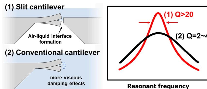
**Figure 1.** Schematic illustration of slit cantilever compared to the conventional structure of cantilever sensors in liquid environment and a conceptual diagram showing an enhanced quality-factor of the slit cantilever by reducing viscous damping due to formation of the air-liquid interface.
