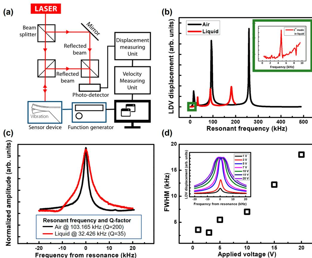
**Figure 3.** Characterization of resonating slit cantilever in air and liquid conditions. (a) An optical measurement setup of the slit cantilever sensor; (b) Measurement of first ~third mode resonant frequencies in air and distilled water; (c) Direct comparison of an identical mode resonance peak between air and liquid phases; (d) Optimization of an induced voltage toward the PZT self-actuating layer.
