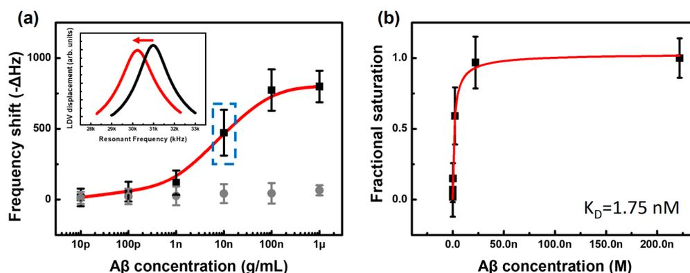
**Figure 4.** Quantification of  $A\beta_{42}$  peptide as a target analyte using the slit cantilever. (a) Responses of resonant frequency vs. logarithmic concentration of analytes (black square) and negative control with PSA protein (grey circle); (b) Estimation of the dissociation constant of specific recognition by fitting the thermodynamic isotherm model.
