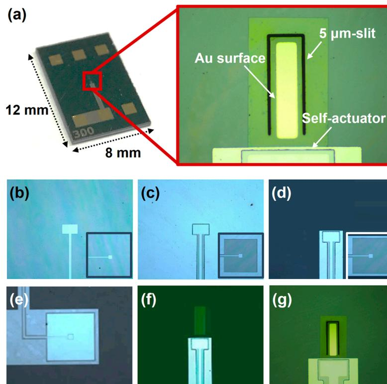
**Figure 2.** Optical images of the slit cantilever and fabrication process (a) a single die of the slit cantilever sensor and fabrication details for (b) upper Pt etching; (c) PZT wet-etching; (d) bottom Pt etching; (e) Au contact pad formation; (f) backside-Si bulk etching; and (g) biological active layer formation and cantilever releasing.
