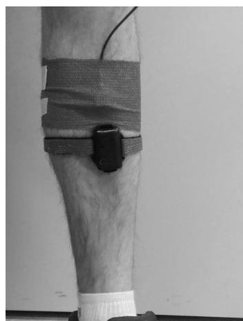
**Figure 3.** Attachment method of the IMU and the reference sensor on the subject's leg.
