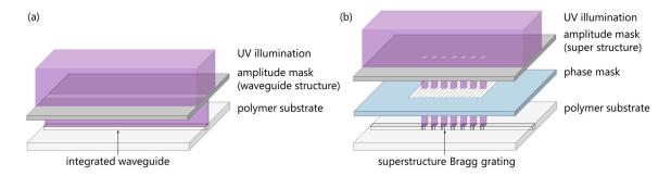
**Figure 3.** Schematic illustration of the setup (vertically exploded assembly drawing) for the fabrication of superstructure Bragg gratings by successively writing (a) an integrated waveguide and (b) a superstructure Bragg grating (masks and polymer substrate are in contact).
