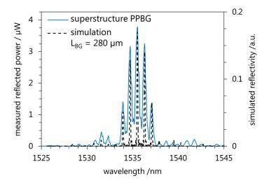
**Figure 5.** Measured reflected spectrum of the fabricated superstructure PPBG in comparison with a simulation based on  $L_{BG}$  being 280  $\mu$ m.
