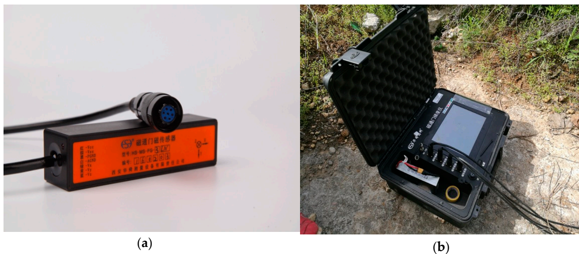
Figure 15. (a) Three-component fluxgate sensor of HS-MS-FG-3-LN; (b) Data acquisition card of NI 9239.
