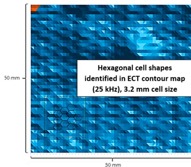
**Figure 9.** ECT core evaluation with identified cell geometries (25 kHz).
