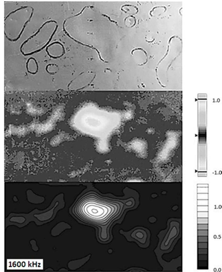
**Figure 5.** Damage region (top); 3D scanning deviation map (middle); 1600 kHz ECT contour map (bottom).
