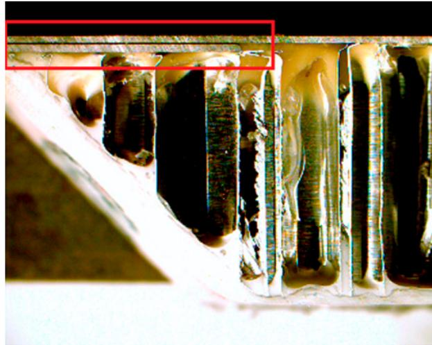
**Figure 8.** Second layer of aluminum identified under top face sheet near top of damage region close to panel flange.
