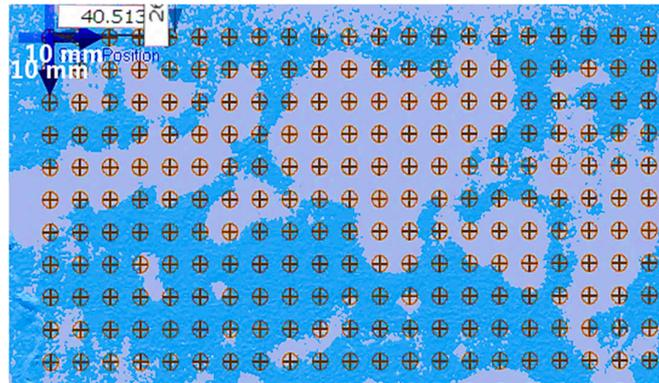
**Figure 3.**  $11 \times 21$  grid of comparison points for damage region as evaluated within 3D scanning software; blue patterned background is 3D scan point cloud data.
