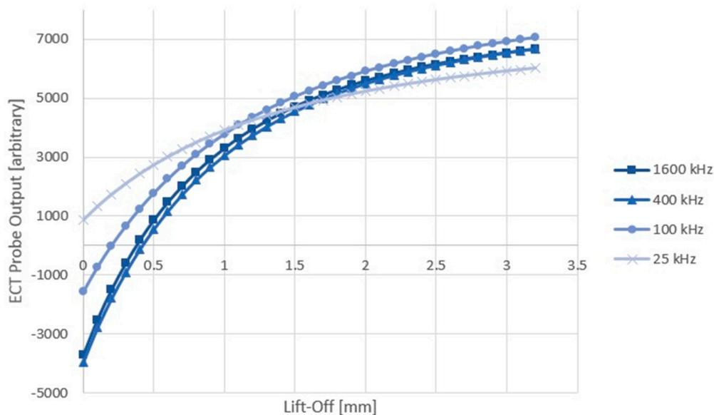
**Figure 2.** Eddy current testing (ECT) calibration curves at various frequencies; probe output vs. lift-off (mm).
