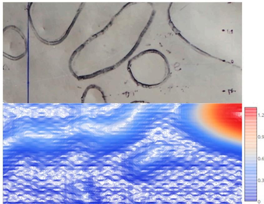
**Figure 11.** ECT core evaluation; panel surface (**top**) and ECT results plotted at 0.0015 mm contour step size (**bottom**) (25 kHz).
