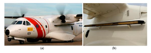
**Figure 1.** (a) Aircraft belonging to Spanish government used to acquire SAR images; (b) Detail of SLAR Terma-sensor antenna, which are 12 ft in dimension.
