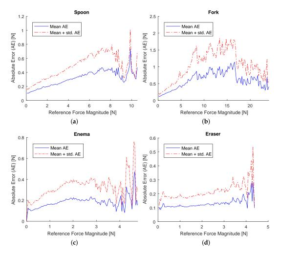
**Figure 7.** Absolute force error magnitude of approximated signals over the measured force magnitudes for four datasets. (a) Absolute error for Spoon dataset; (b) Absolute error for Fork dataset; (c) Absolute error for Enema dataset; (d) Absolute error for Eraser dataset.
