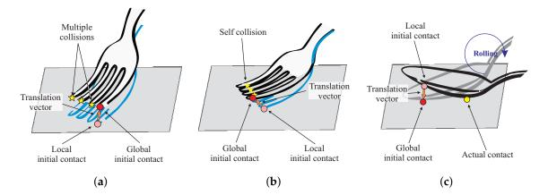
**Figure 2.** Complex contact deformation: our data-driven model provides a non-linear input-output mapping that allows simulating the following deformations (**a**) multiple-contact; (**b**) self-collision; and (**c**) rolling-contact.
