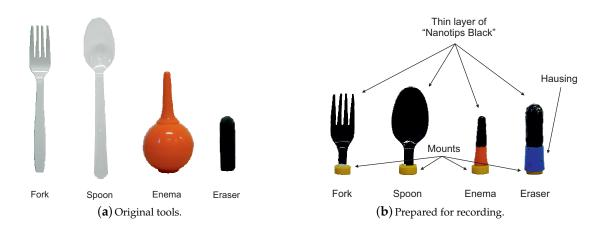
**Figure 5.** A set of real tools for evaluation: (**a**) illustration of original tools; and (**b**) modified versions of tools prepared for numerical and psychophysical experiments.
