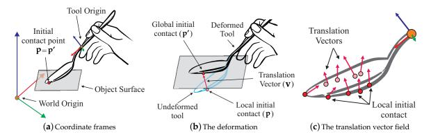
Figure 1. Descriptions of the model input space: (a) the input space is defined with respect to the origin of a tool; (b) a six-dimensional input vector consists of a position of an initial contact  $\mathbf{p}$  and a translation vector,  $\mathbf{v}$  that describes the state of deformation; (c) A set of recorded input vectors are used in interpolation, and the force response is approximated at the tool's origin during rendering.
