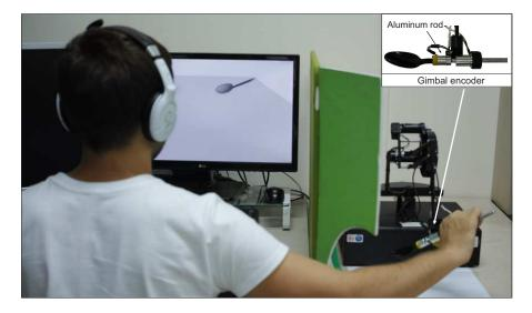
**Figure 8.** Hardware setup for the experiment. A tool is attached to the gimbal encoder (see top-right) during interaction with a real tool, and detached when the subject interacts with a virtual tool.
