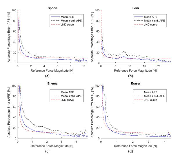
**Figure 6.** Relative error of the approximated signals for four datasets. The value of the relative error is expressed by absolute percentage error, which denotes the ratio of the force error magnitude to the magnitude of the reference force. The JND curve was computed based on data from psychophysical study in [50]. (a) Relative error for Spoon dataset; (b) Relative error for Fork dataset; (c) Relative error for Enema dataset; (d) Relative error for Eraser dataset.
