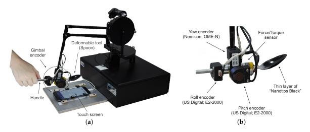
**Figure 4.** Data recording setup. A user holds the handle of the device and presses the tool to surface of the touchscreen. Data from the tool deformation is recorded when the tool is in contact with the touchscreen. (**a**) Recording hardware; (**b**) Gimbal encoder.
