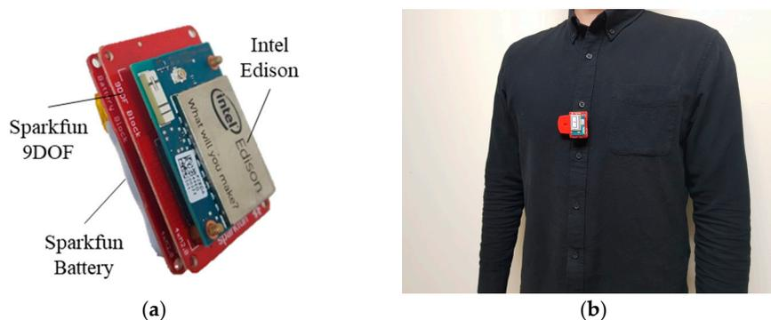
**Figure 1.** Overview of the apparatus. (a) Packaging of the Intel Edison, Sparkfun 9DOF, and Sparkfun Battery; (b) Appearance of the apparatus when worn by participant.
