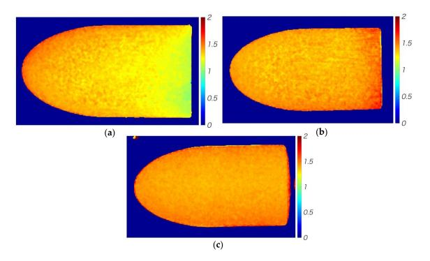
**Figure 6.** Luminescence ratio distributions on the test models. (**a**) Static dipping; (**b**) Convectional dipping; (**c**) Rotational dipping.
