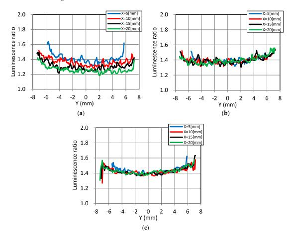
**Figure 10.** Luminescence ratio plots along the *Y*-axis (circumference direction). (**a**) Static dipping; (**b**) Convectional dipping; (**c**) Rotational dipping.
