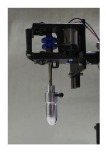
Figure 4. Rotational mechanism for rotational dipping.
