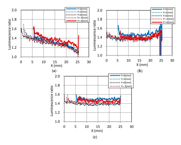
**Figure 8.** Luminescence ratios along the X-axis (longitudinal direction). (**a**) Static dipping; (**b**) Convectional dipping; (**c**) Rotational dipping.
