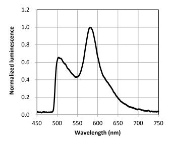
**Figure 5.** Emission spectra of two-color TSP consists of rhodamine B and fluorescein excited by a 405 nm laser.
