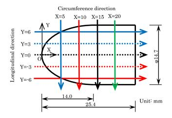
Figure 7. Position of the luminescence ratio profile extraction.
