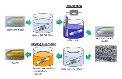
Figure 2. Schematic of the test model preparation.
