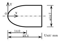
Figure 1. Shape of test model.
