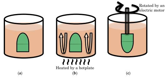
**Figure 3.** Schematic depictions of dipping methods. (**a**) Static dipping; (**b**) Convectional dipping; (**c**) Rotational dipping.
