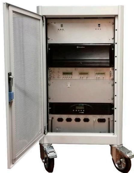
**Figure 1.** The time domain near infrared spectroscopy (TD NIRS) medical device.
