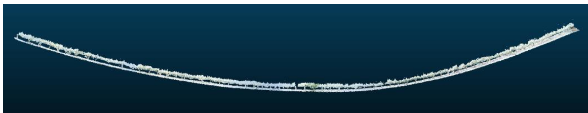
Figure 2. 3D reconstruction of a woody crop row in which the drift problem is observed.
