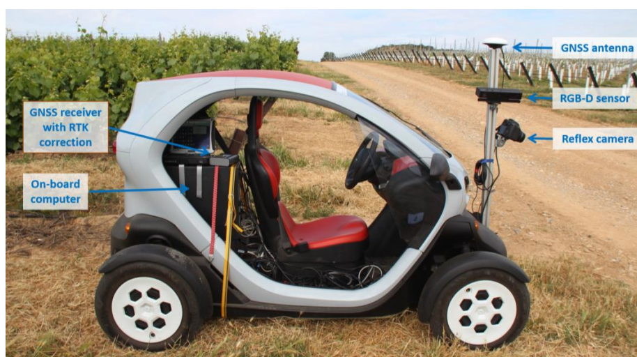
Figure 1. Field platform and on-board equipment.
