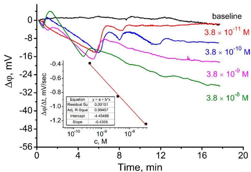
**Figure S4.** Real time signal of the ISFET (in  $\Delta\phi$ ) during Bsm DNA polymerase reaction in homogenous solution in Bsm buffer initiated (30–40 s) by addition of DP at different concentration (final concentration are marked on the picture); Slope ( $\Delta\phi/\Delta t$ ) dependence on DP concentration calculated from real time signal curves is presented as insert. Reaction conditions: 0.2 mM dNTP, 0.05 pmol/ $\mu$ l FP, 1.6 pmol/ $\mu$ l PR, 0.1 U/ $\mu$ l BSM DNA polymerase.
