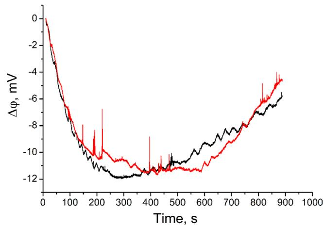
**Figure S5.** Real time signal of the ISFET (in  $\Delta\phi$ ): black line—Selection buffer with 0.2 mM dNTP, 0.05 pmol/ $\mu$ l FP, 1.6 pmol/ $\mu$ l PR, 0.1 U/ $\mu$ l BSM DNA polymerase, red line—Selection buffer with 0.2 mM dNTP, 0.05 pmol/ $\mu$ l FP, 1.6 pmol/ $\mu$ l PR, 0.1 U/ $\mu$ l BSM DNA polymerase during polymerase reaction initiated by addition of DP (35 s) at concentration of  $3 \times 10^{-8}$  M.
