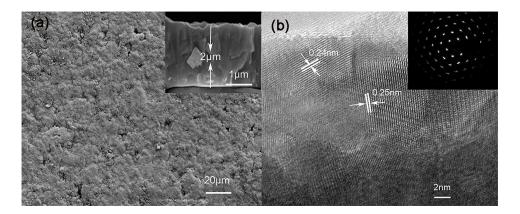
Figure 3. (a) SEM images of ZnO film; and (b) HRTEM and SAED images of ZnO film.
