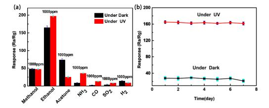
**Figure 7.** (**a**) Responses to various gases and (**b**) the long-term stability for seven days toward 100 ppm ethanol of the ZnO film sensors under dark and under UV light illumination.
