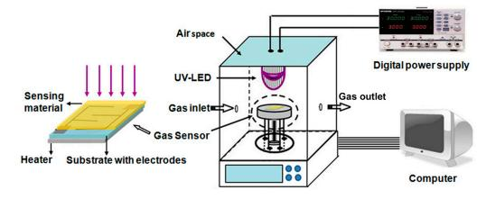
Figure 1. The schematic structure of the gas sensor and gas sensing measurement system.
