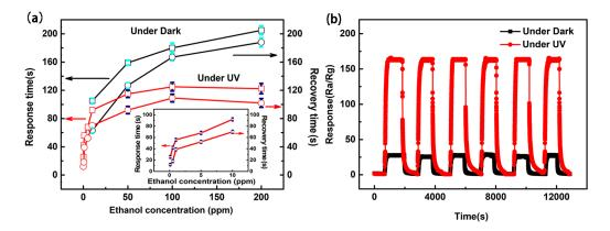
**Figure 6.** (a) The response and recovery times to different concentrations of  $C_2H_5OH$  and (b) six cycles of response curves to 100 ppm  $C_2H_5OH$  of the ZnO film sensors under dark and under UV light illumination.
