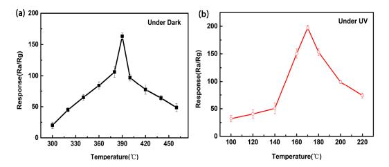
**Figure 4.** Response of the ZnO film sensor to 1000 ppm ethanol (**a**) under dark and (**b**) under UV light illumination as a function of the operating temperature.
