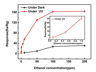
**Figure 5.** Response of the ZnO film sensor to different concentrations of  $C_2H_5OH$  from 0.1 to 200 ppm under dark and under UV LED activation.
