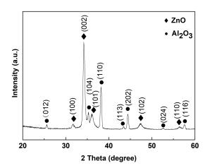
Figure 2. XRD pattern of the synthesized ZnO film deposited by RF magnetron sputtering.
