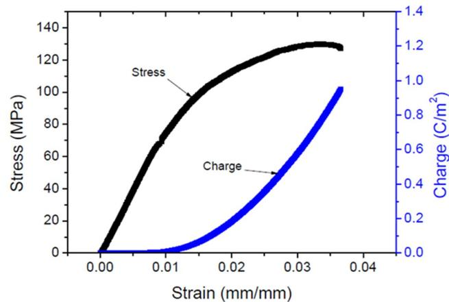
**Figure 5.** Stress–strain and charge curves of cellulose ZnO hybrid nanocomposite (CEZOHN) [38].
