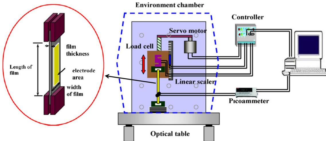
Figure 2. Schematic of piezoelectric charge constant measurement based on direct piezoelectricity [31].
