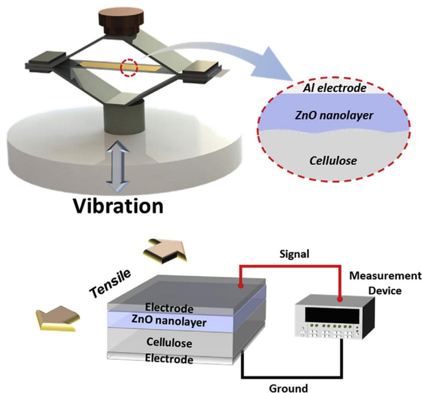
**Figure 20.** Cymbal type vibration energy harvester [27].
