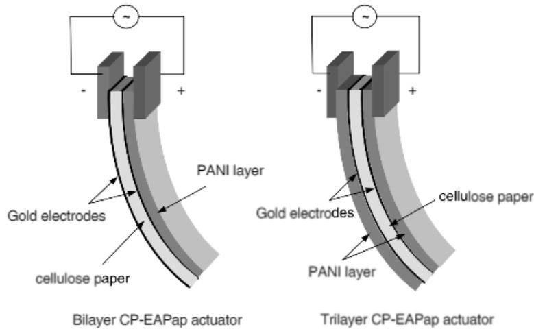
Figure 9. Schematic of bi-layer and tri-layer CP-EAPap actuators [51]. (PANI-polyaniline).
