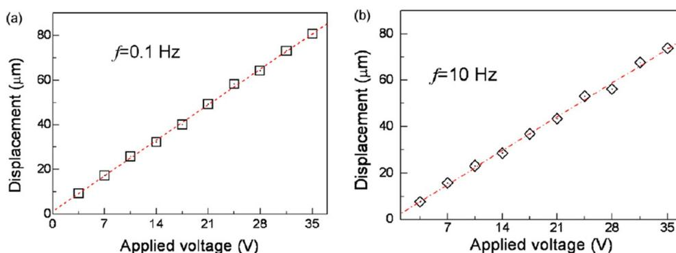
**Figure 7.** Plots of the bending displacement versus the applied voltage ( $V_{amp}$ ) at the frequencies of (a)  $f = 0.1$  Hz and (b)  $f = 10$  Hz [47].
