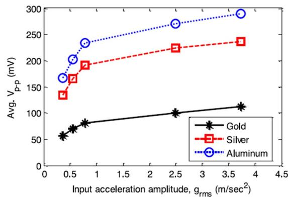
**Figure 18.** Variation of the average  $V_{p-p}$  against the input acceleration amplitude ( $g_{rms}$ ) for three parallel connected electrodes with an area of 1200 mm<sup>2</sup> [81].
