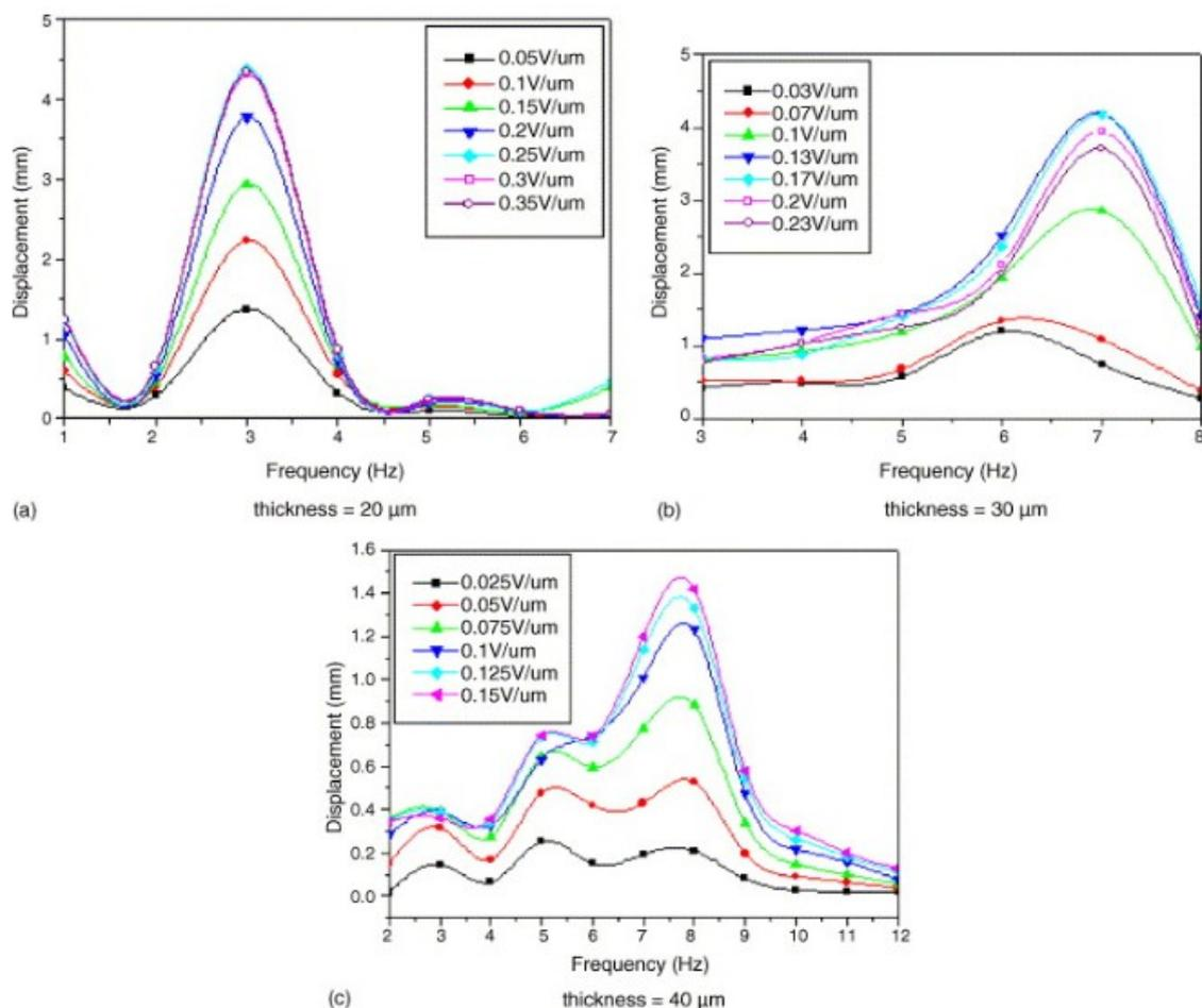
Figure 13. (a–c) Tip displacements of EAPap actuators with thickness variation [32].
