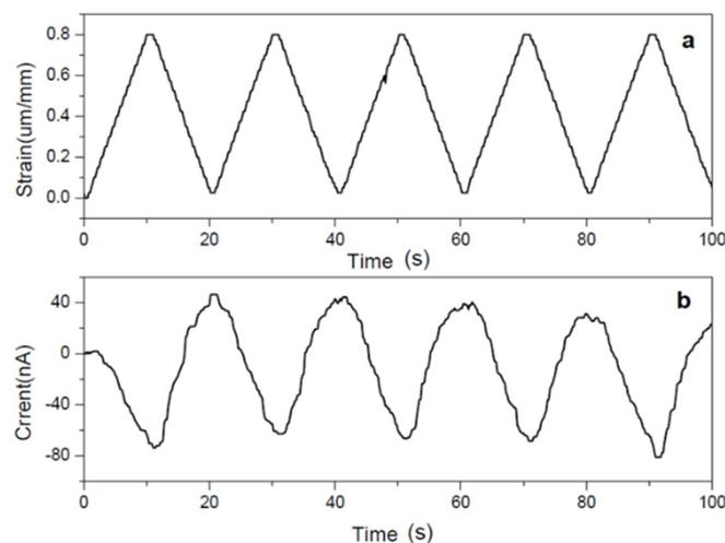
**Figure 6.** Stretching mode strain sensor: (a) stretching strain and (b) sensor signal [38].
