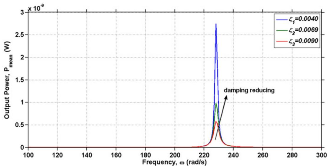
**Figure 15.** Mean power output of the EAPap-based energy harvester for a range of frequencies in different damping ratios [79].
