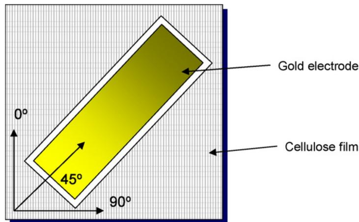
Figure 3. Orientation of cellulose film and schematic of EAPap [31].
