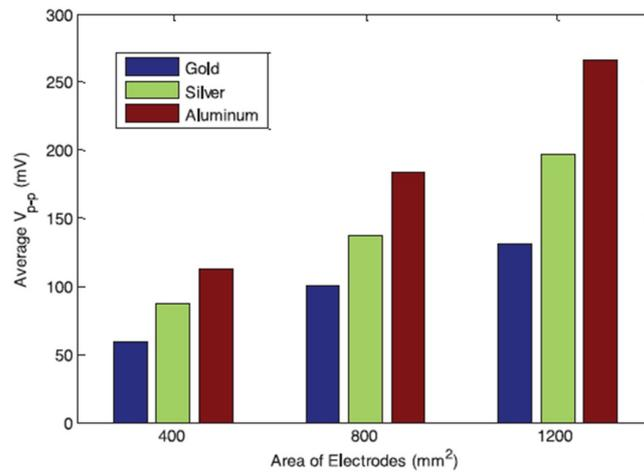
**Figure 17.** Average peak to peak open circuit voltage output for 400, 800, and 1200 mm<sup>2</sup> gold, silver, and aluminum electrode-coated EAPap [81].
