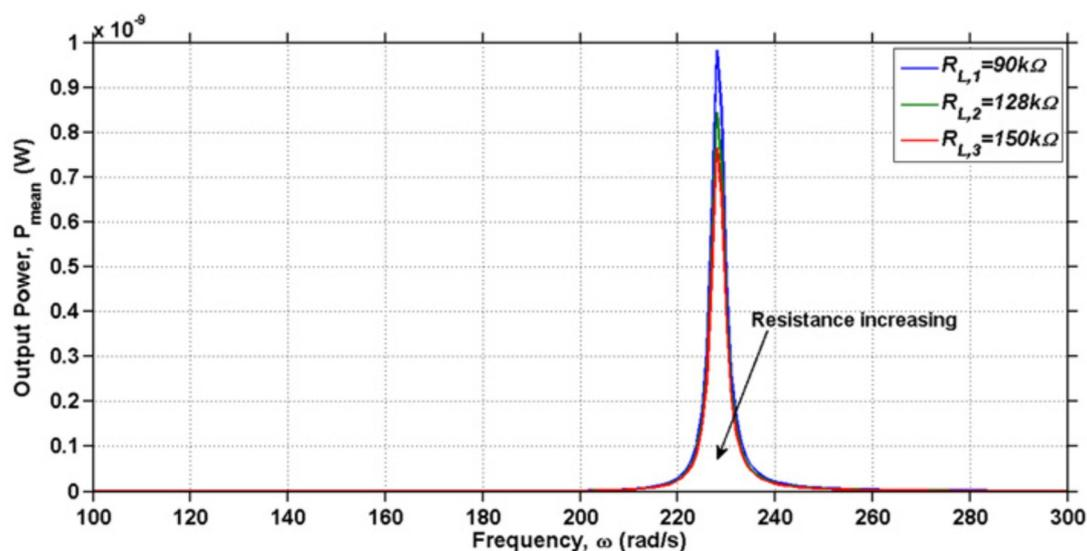
**Figure 14.** Mean power output of the EAPap-based energy harvester for a range of frequencies with different external resistive loads [79].
