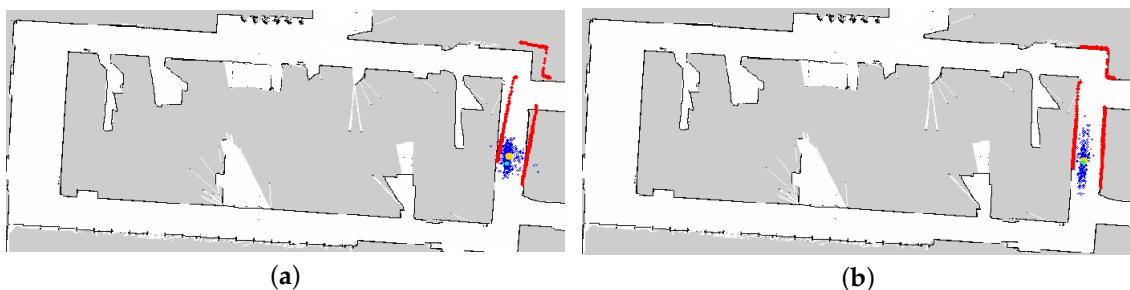
**Figure 11.** Self-correction of local pose tracking. (a) The position deviated when the robot rotated. (b) The robot corrected the pose automatically with HPFL.
