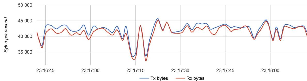
Figure 21. Bandwidth usage for a router with Configuration 3.
