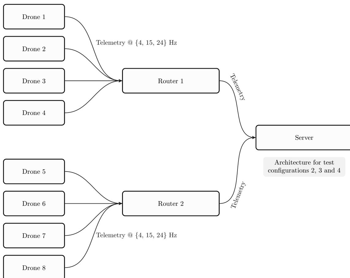
**Figure 16.** Test architecture for configurations.
