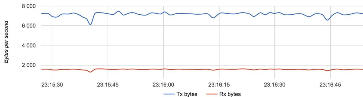
Figure 20. Bandwidth usage for a drone with Configuration 3.
