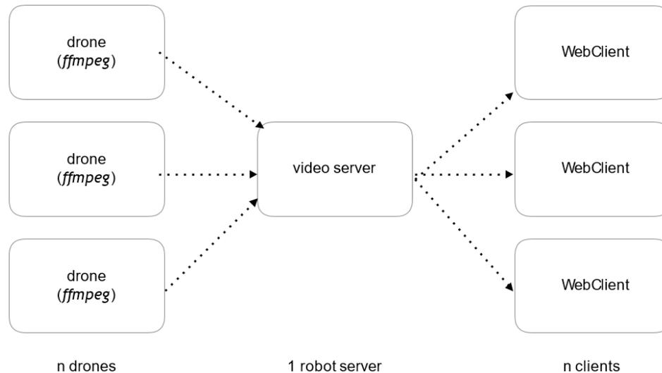
Figure 15. Multimedia transmission architecture.
