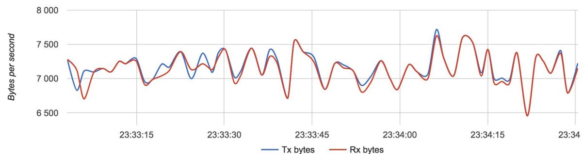
**Figure 18.** Bandwidth usage for a router with Configuration 1.
