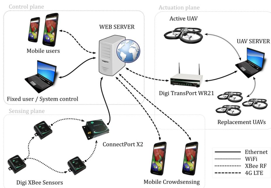
Figure 5. Functional description of the proposed architecture.
