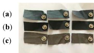
**Figure 3.** The shape of textile electrode used for ECG measurements; (a) 100% cotton; (b) cotton/Lycra; (c) silver-plated.
