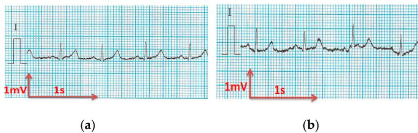
**Figure 13.** ECG signal obtained by cotton/Lycra electrodes with 11.9 wt.% PEDOT:PSS; (a) before washing; (b) after 50 washing cycles.
