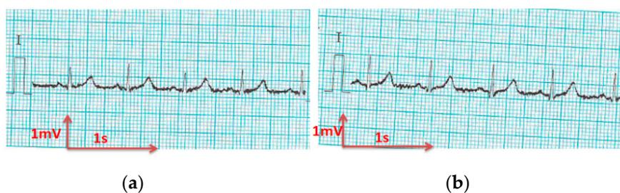
**Figure 14.** ECG signal obtained by silver-plated electrodes: (a) before washing; (b) after 50 washing cycles.
