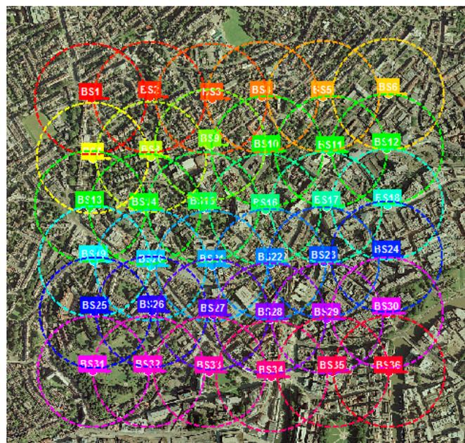
**Figure 2.** Base station deployment showing the coverage radius.
