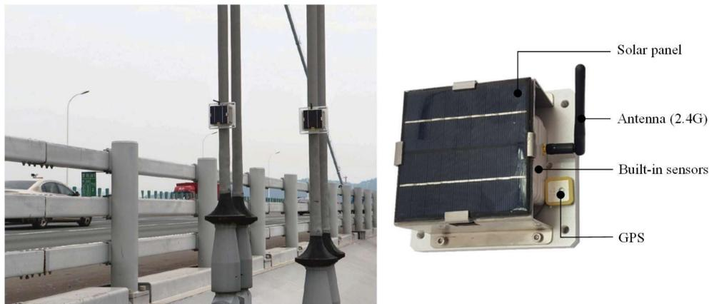
**Figure 5.** Wireless sensor nodes with two-axis MEMS accelerometers attached on hanger cables.
