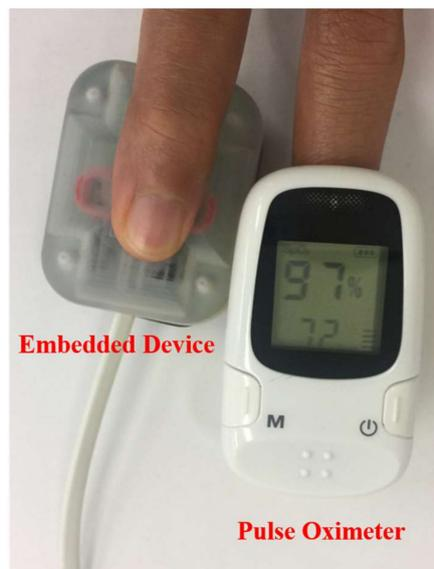
**Figure 7.** Heartbeat measurement setup with the subject's hand.
