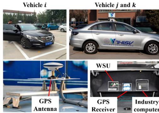
**Figure 5.** Experimental vehicles. WSU, GPS Receiver, and industry computer are installed in the trunk of each test vehicle.
