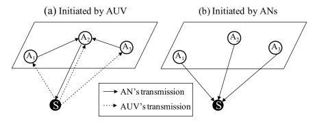
Figure 1. Communication scheme for the ranging.
