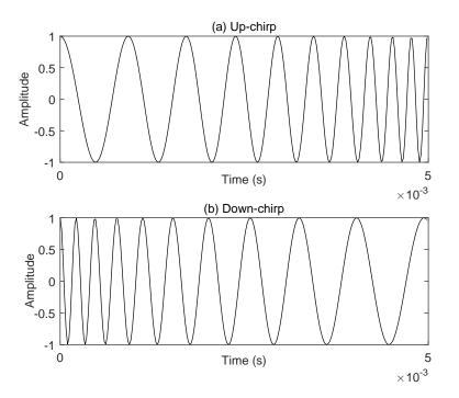
Figure 5. An example of HFM signal, assuming that T is 5 ms, and the used frequency band is [1, 5] kHz.
