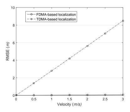
Figure 9. The impact of MAC delay and AUV movement on the localization, network size is 300 m.
