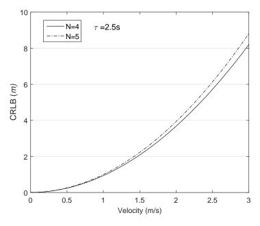
**Figure 4.** The CRLB with respect to the AUV's velocity, network size:  $1500 \times 1500 \times 1500$  m<sup>3</sup>, initial position of the AUV: (750, 750, 750).
