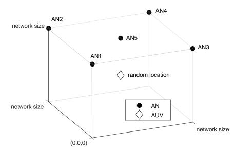
**Figure 6.** Network topology: Total 5 ANs are deployed on the surface and the location of AUV is randomly selected. The network size is two cases, 300 m and 1500 m.
