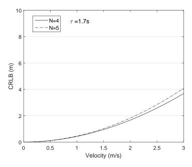
**Figure 3.** The CRLB with respect to the AUV's velocity, network size:  $300 \times 300 \times 300$  m<sup>3</sup>, initial position of the AUV: (150, 150, 150).
