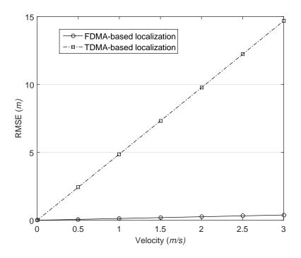
Figure 10. The impact of MAC delay and AUV movement on the localization, network size is 1500 m.
