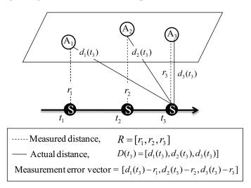
**Figure 2.** The impact of MAC delay and the AUV movement on the localization initiated by ANs' transmission.
