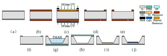
Figure 1. Fabrication process of the first silicon wafer. (a-j) Steps 1-10.
