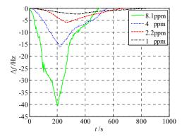
Figure 7. Real-time resonant frequencies for ethanol vapor.
