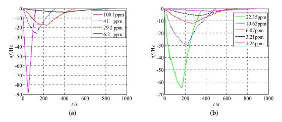
**Figure 8.** Real-time resonant frequencies for hydrogen gas and ammonia gas. (a) Hydrogen gas; (b) ammonia gas.
