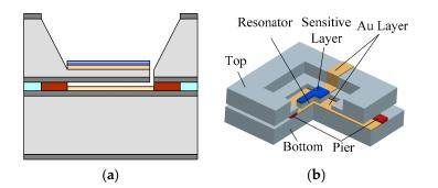
Figure 3. Two silicon wafers bonded. (a) Schematic diagram of cross section; (b) 3D diagram.
