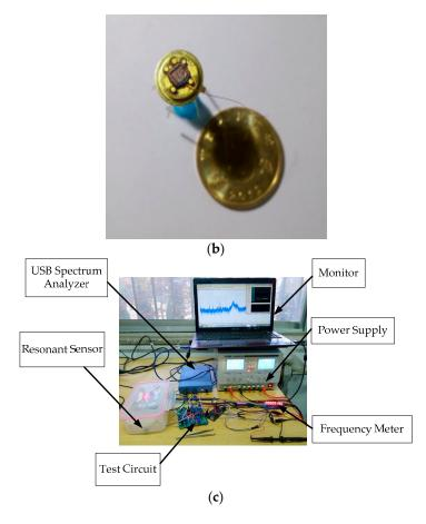
Figure 5. Micro-resonant gas sensor and its test system. (a) The cantilever; (b) the micro-resonant gas sensor; (c) the test system.
