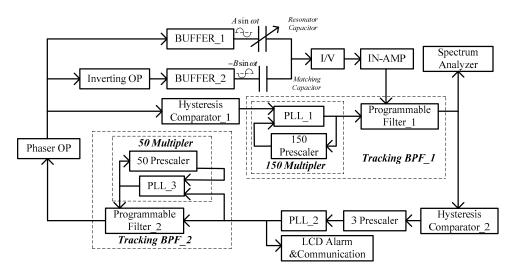
Figure 4. Block diagram of the self-exciting closed loop system.
