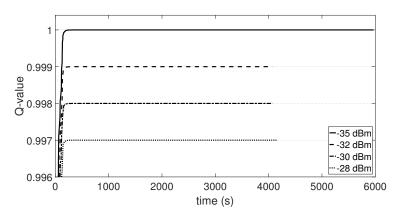
**Figure 7.** Normalized Q-value of the single agent in a network of two nodes (2 m node distance) and average inter-arrival time of 25 ms, where the trend is focused on the lowest transmission power levels.
