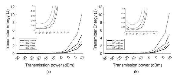
**Figure 14.** Transmit energy consumption, zooming on the lower values, of the homogeneous network with eight nodes and d equal to: 2 m (**a**); and 4 m (**b**).
