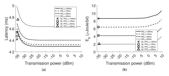
**Figure 8.** Performance in WSN with 2 nodes during the testing period (2 m node distance): average latency (**a**); and energy consumption per bit (**b**).
