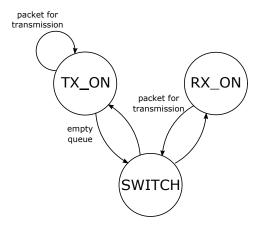
Figure 6. Finite state machine of the energy model.
