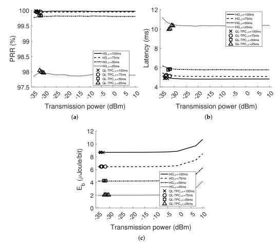
**Figure 11.** Performance in WSN with eight nodes during the testing period (2 m node distance): average PRR (**a**); average latency (**b**); and energy consumption per bit (**c**).
