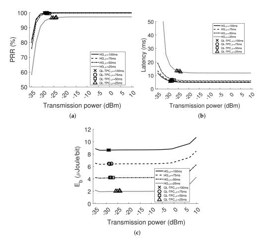
**Figure 12.** Performance in WSN with eight nodes during the testing period (4 m node distance): average PRR (**a**); average latency (**b**); and energy consumption per bit (**c**).
