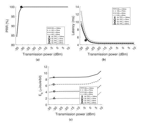
**Figure 9.** Performance in WSN with two nodes during the testing period (4 m node distance): average PRR (**a**); average latency (**b**); and energy consumption per bit (**c**).
