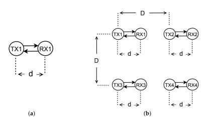
**Figure 5.** WSNs with Manhattan grid topology: (**a**) single agent—one wireless communication without interference; and (**b**) multi-agent—four interfering pairs.
