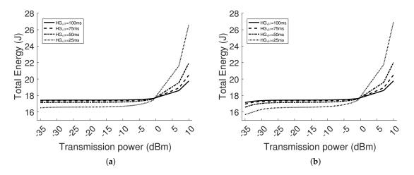
**Figure 15.** Total energy consumption of the homogeneous network with eight nodes and *d* equal to:  $2 \text{ m}(\mathbf{a})$ ; and  $4 \text{ m}(\mathbf{b})$ .
