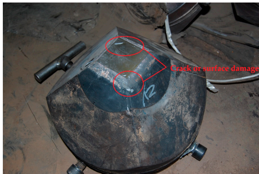
Figure 6. The cracked anvil.
