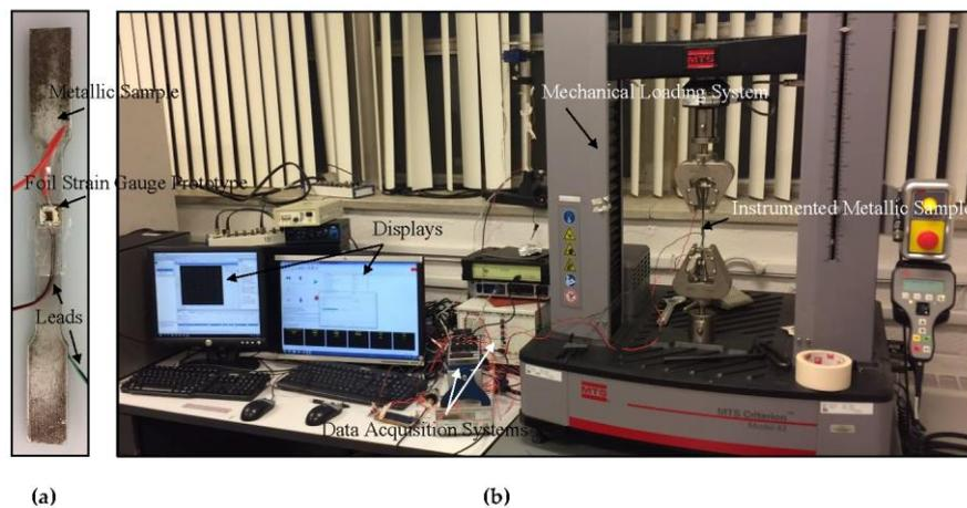
**Figure 7.** (a) Optical image of the dog-bone steel sample instrumented with a foil strain gauge prototype; (b) Experimental setup used to calibrate foil strain gauge prototypes.
