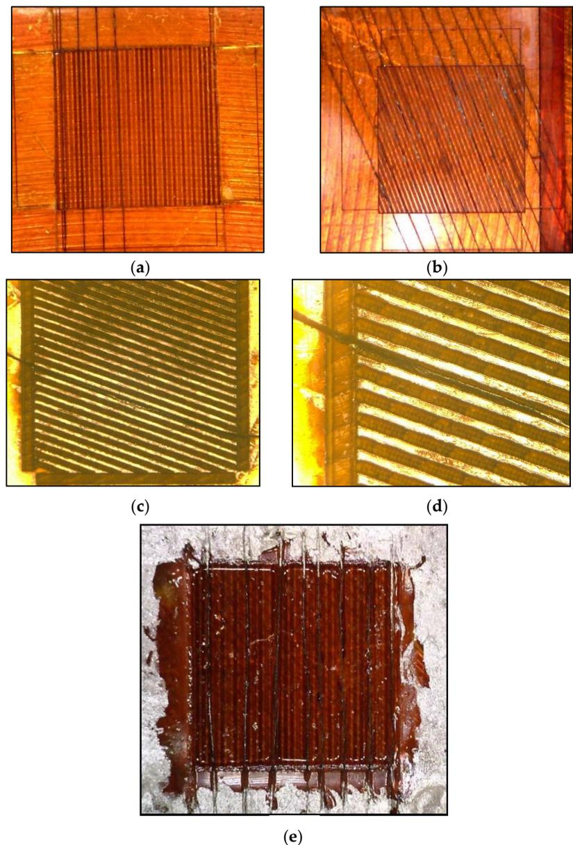
**Figure 6.** Optical images of the foil strain gauge prototypes: (a) Substrate with several CNT yarns placed in the grooves at  $0^\circ$ -inclination; (b) Substrate with several CNT yarns placed in the grooves at  $70^\circ$ -inclination. (c) Substrate with a CNT yarn placed in the groove; (d) Close-up of the substrate with a single CNT yarn placed in the groove; (e) Complete gauge showing CNT yarns in the grooves, adhesive layer on the gauge area, and conductive silver on the electrodes.
