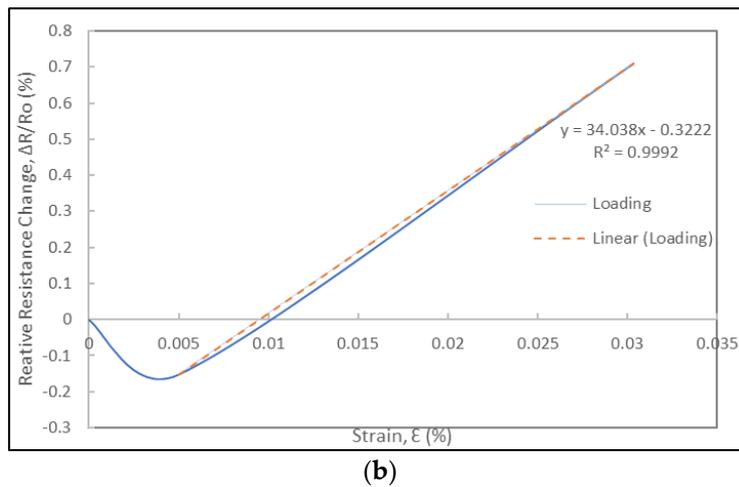
**Figure 9.** Electromechanical response of the same foil strain gauge prototype under subsequent cyclic loading at a displacement rate of 300 μm/min: (a) Strain and relative resistance change histories during three loading-unloading cycles. (b) Relative resistance change versus strain curve of first loading cycle and corresponding gauge factor.
