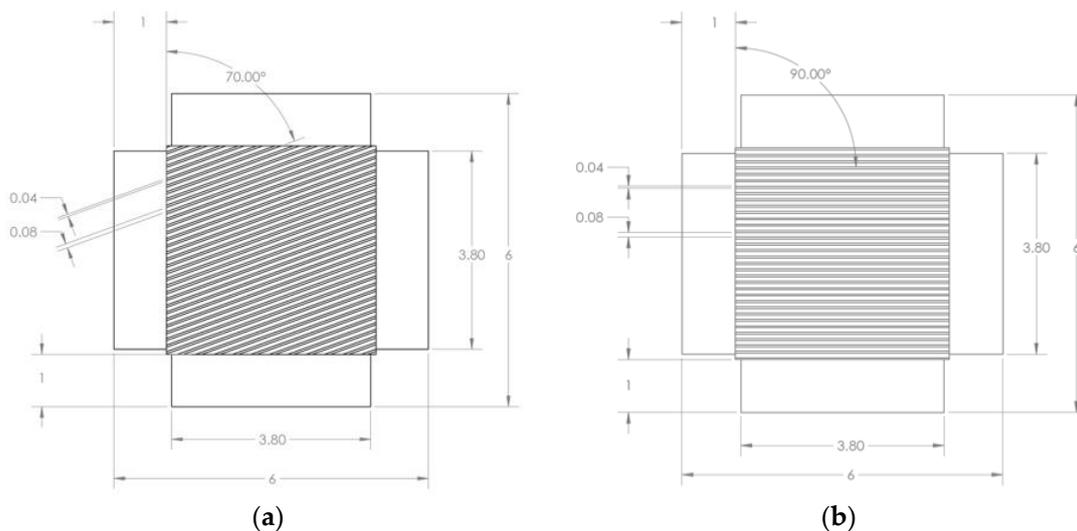
**Figure 4.** Schematics of the foil strain gauge substrates showing the grooves. (a) Grooves oriented at  $70^\circ$ ; (b) Grooves oriented at  $0^\circ$  or  $90^\circ$ . Dimensions are in mm.
