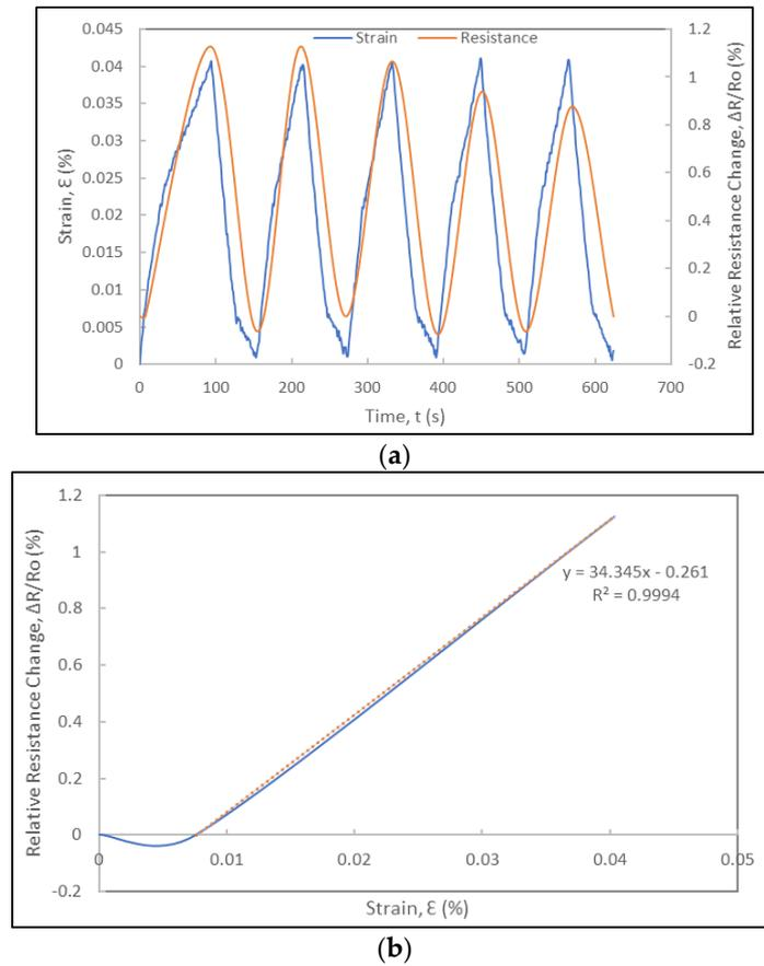
**Figure 8.** Electromechanical response of a foil strain gauge prototype under cyclic loading at a displacement rate of  $300 \mu\text{m}/\text{min}$ : (a) Strain and relative resistance change histories during five loading-unloading cycles; (b) Relative resistance change versus strain curve of first loading cycle and corresponding gauge factor.
