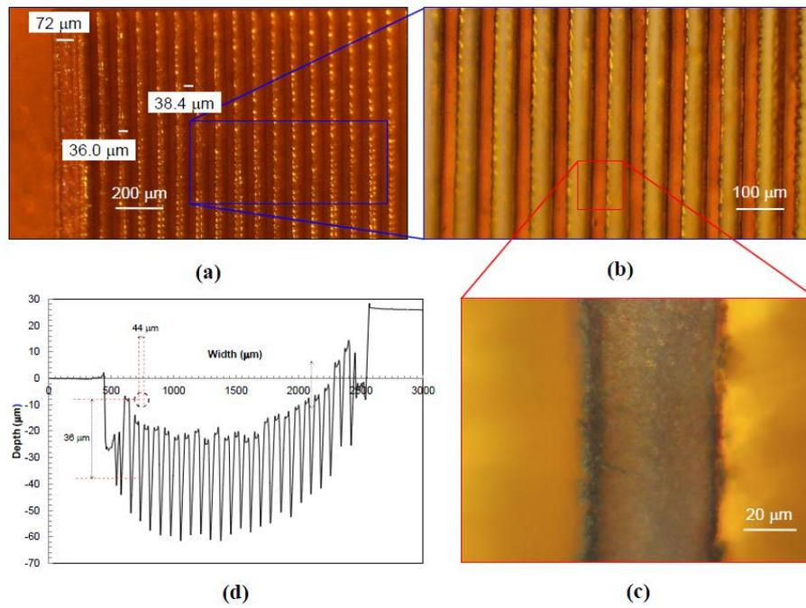
**Figure 3.** Foil strain gauge substrate with grooves oriented at  $0^\circ$ . (a) Optical image of substrate including one border for the electrode; (b) Close-up optical image of substrate; (c) Close-up optical image of a single groove; (d) Profilometer data indicating the width and depth of each groove.
