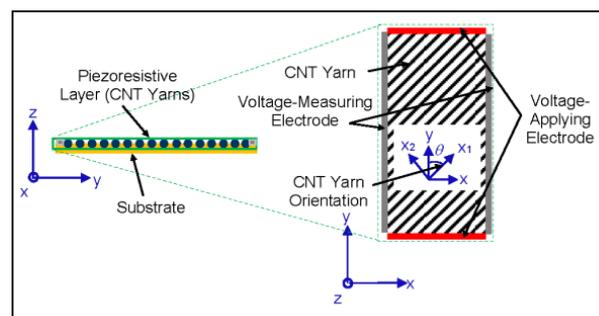
**Figure 1.** Schematic of cross-section of the foil strain gauge sensor comprising CNT yarns. Inset: top schematic view of the arrangement of the CNT yarns in a unidirectional configuration [65].
