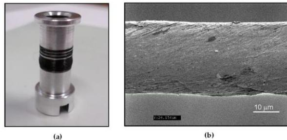
**Figure 2.** (a) Optical image of a spool with the CNT yarn; (b) Scanning Electron Microscope (SEM) image of a one-thread CNT yarn.
