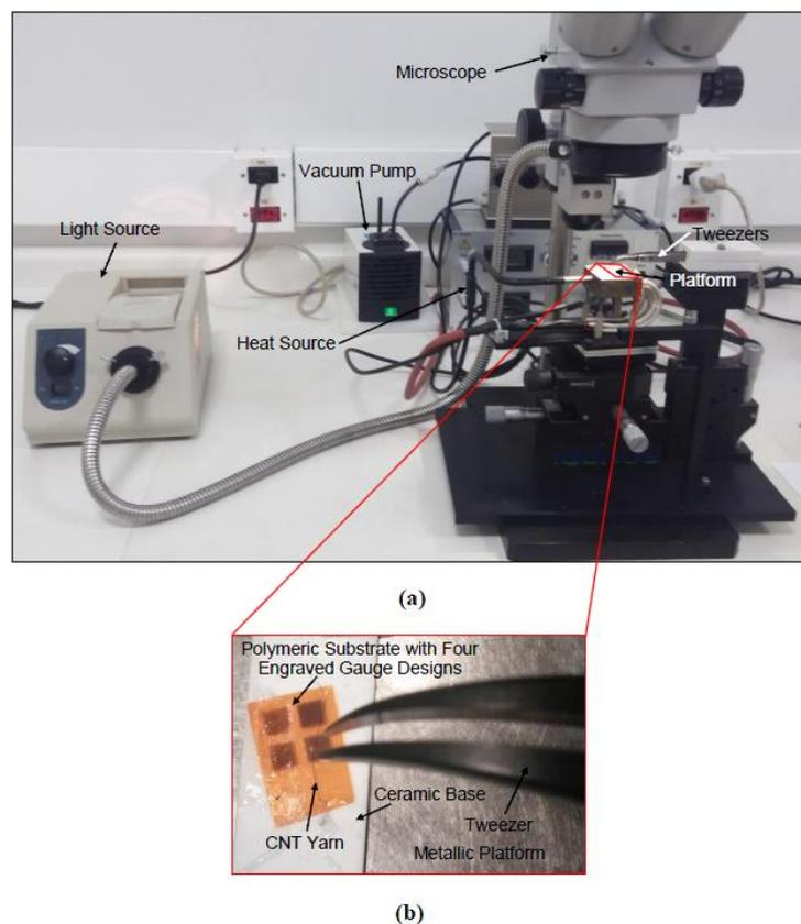
**Figure 5.** (a) Optical image of the experimental setup used initially to place the CNT yarns in the substrate consisting of a microscope with an adjustable platform and a vacuum connection; (b) Close-up optical image of the adjustable platform.
