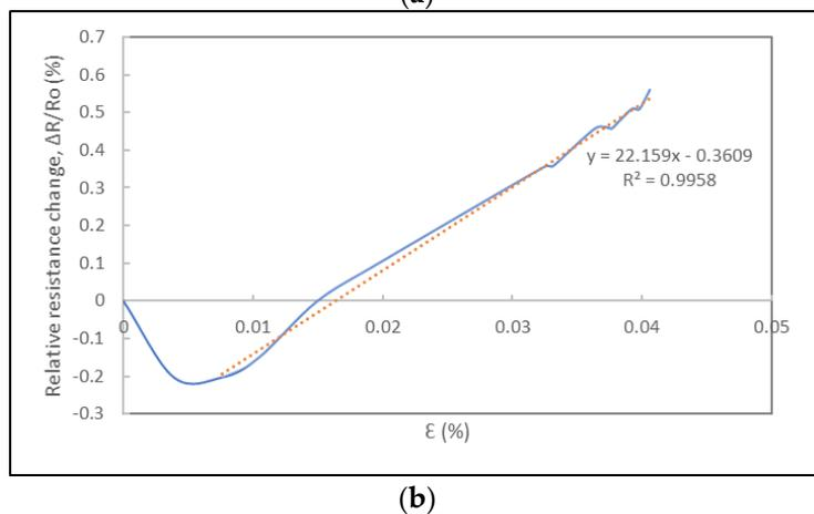
**Figure 10.** Electromechanical response of foil strain gauge prototype under cyclic loading at displacement rate of 150 μm/min: (a) Strain and relative resistance change histories during one cycle; (b) Relative resistance change versus strain curve of loading cycle and corresponding gauge factor.
