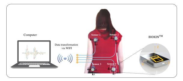
**Figure 1.** Experiment setup: Four BioKin<sup>TM</sup> sensors are attached on the back, connected to computer via wifi.
