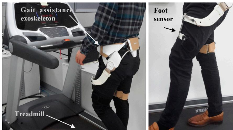
Figure 7. Experimental setup with a treadmill.
