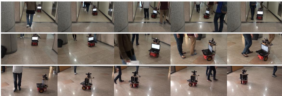
**Figure 11.** Snapshots from a real autonomous robot navigation experiment using the proposed motion model and motion controller in an L-shape lobby.
