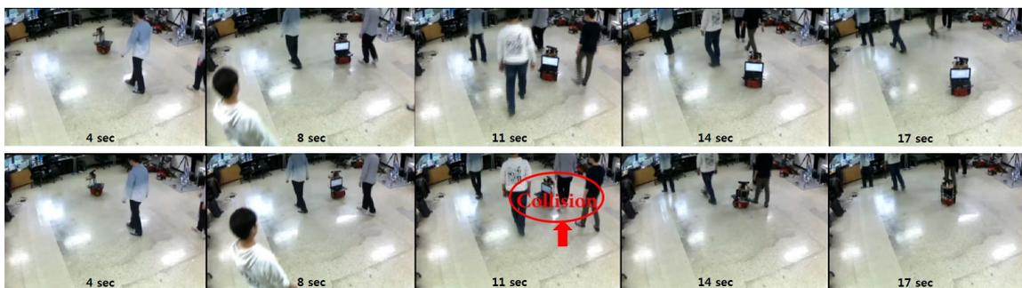
**Figure 10.** Snapshots from a motion control experiment in a laboratory with four moving pedestrians using: FactGP<sub>C</sub> (top); and GP-MC (bottom) .
