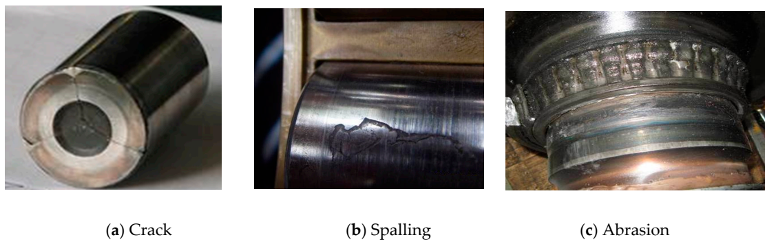
Figure 1. Different railway axle bearing defects.
