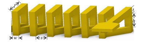
Figure 2. The geometric structure parameters diagram of the micro-inductor coil.
