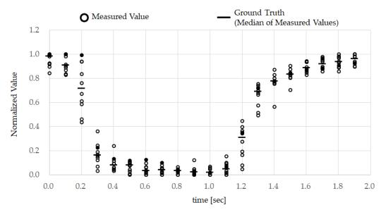
**Figure 5.** Ground truth obtained from subject A: the subject repeated TEMPO ten times, while the movement of the external acoustic meatus was measured by the earphone-type sensor. The obtained data was normalized, and the median values from the normalized data from each time were extracted and used as the ground truth as described in Section 3.2.
