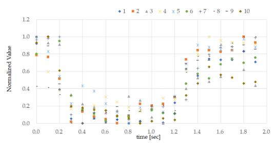
**Figure 7.** Measured values of person A while walking. The result is obtained by normalizing the measurement values of the earphone-type sensor when person A performs the TEMPO 10 times while walking. These measurement values were obtained from the experiment discussed in Section 3.3.
