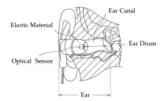
**Figure 4.** Measurement principle for changes in the shape of the ear canal. The earphone-type sensor receives the light emitted from the optical distance sensor that is reflected back by the eardrum and ear canal. During movement of the tongue, the shape of the ear canal changes, which alters the distance between the optical distance sensor and the eardrum and ear canal. The amount of light received changes over time in association with this change in distance.
