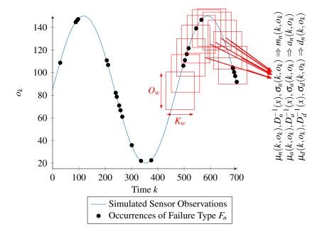
**Figure 9.** Sliding window approach for identifying time- and value-correlations for a failure type  $F_n \in \mathcal{F}_2$ .
