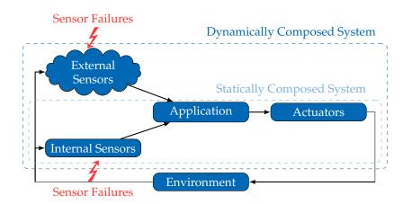
Figure 1. Basic control loop and components of statically composed systems and dynamically composed systems.
