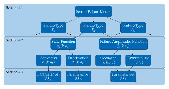
Figure 4. Hierarchical overview on the generic failure model.
