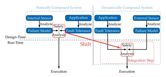
Figure 2. Comparison of safety analysis in statically composed systems and dynamically composed systems.
