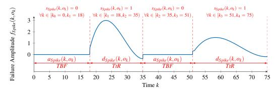
Figure 6. State function for modeling an exemplary Spike failure type with two occurrences.
