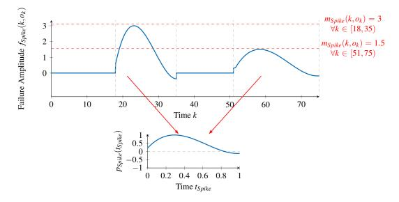
**Figure 5.** Example of a Spike failure type with two occurrences, modeled through a failure pattern and a stochastic function.
