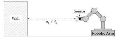
Figure 10. Evaluation setup to acquire real sensor data from a Sharp GP2D12 infra-red distance sensor.
