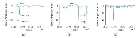
**Figure 13.** Comparing 140 time steps of failure amplitudes from the Sharp GP2D12 sensor, the generic failure model, and the neural network. (**a**) validation data; (**b**) generic failure model; (**c**) neural network.
