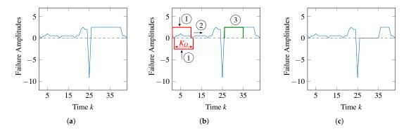
**Figure 8.** Steps for identifying failure types within the first phase of the processing chain. (a) initial failure amplitudes  $f(k, o_k)$ ; (b) step 2 for identifying failure types; (c) step 4 for identifying failure types.
