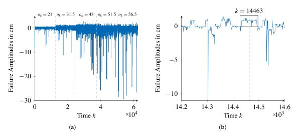
**Figure 11.** Failure amplitudes from the Sharp GP2D12 infra-red distance sensor. (**a**) complete series of failure amplitudes; (**b**) segment of the failure amplitudes for reference distance  $o_k = 31.5$  cm.
