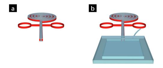
**Figure S5.** Bi-spiral capillary patterns as more compact designs than the serpentine capillary tubes. The overall length of the capillary tube can be extended within a limited space thus enable the detection over a larger pressure range.
