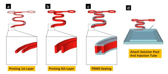
**Figure S1.** Schematic illustration of the manufacturing process of our capillary pressure sensor. (a) Printing 1st and (b) 5th layer directly on temper glass substrate; (c) Seal the top and bottom of the adjacent conductive electrodes to form the capillary conduction channel; (d) Attach solution pool and injection tube to complete the pressure sensor structure.
