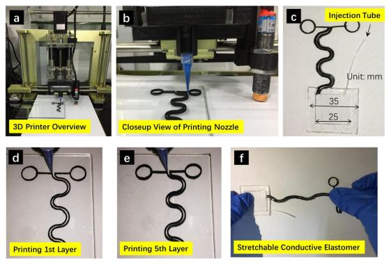
**Figure S2.** (a) Overview of the home-build 3D printer; (b) Close-up view of printing nozzle for extrusion of conductive CNT/PDMS ink; (c) Photograph of a complete pressure sensor with solution pool and injection tube; (d–e) Photographs of printing 1st layer and 5th layer of the elastomer electrode directly on temper glass substrate; (f) Photograph of the capillary electrodes made of conductive elastomer upon stretching.
