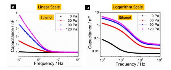
**Figure S4.** The relationship between capacitance and frequency at applied pressure of 0 Pa, 30 Pa, 90 Pa and 120 Pa within 1 KHz - 1 MHz frequency range: (a) linear scale and (b) logarithm scale plot.
