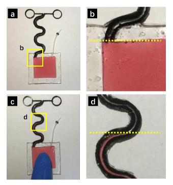
**Figure S3.** Photographs of the pressure sensor (a-b) without and (c-d) with external pressure. The liquid medium levels can be clearly viewed in the enlarged views.
