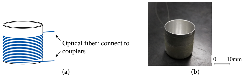
Figure 2. The 3D shaped optical fiber ultrasonic sensor: (a) sketch; (b) photo.
