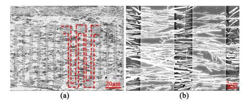
**Figure 4.** FESEM images of the device: (a) ZnO nanowires device with finger shape Au electrodes after the process of nanowire assembly on the Si substrate (red dotted line denotes the finger shape electrodes); and (b) the zoom-in image of the device.
