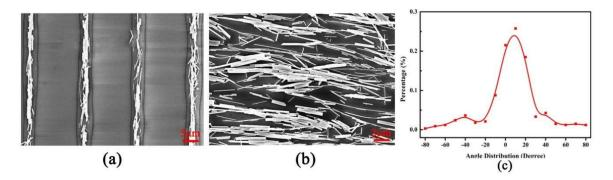
**Figure 3.** (a) FESEM image of four nanowires arrays; (b) the zoom-in image of the first column; and (c) the angle distribution of ZnO nanowire in the first column.
