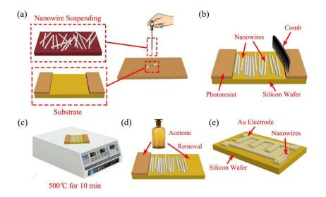
**Figure 2.** Simplified process flow diagram of the assembly of nanowire on the silicon substrate and nanodevice fabrication. (a) Drip a drop of the suspension on the substrate; (b) combing process after 24 h; (c) bake on hot plate for ~10 min at 500 °C; (d) remove the photoresist and not adhered nanowires by acetone; (e) standard electron-beam lithography and metal deposition.
