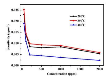
Figure 8. Relationship of sensitivity with respect to concentration of CO at different operating temperatures.
