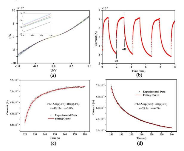
**Figure 5.** Characteristics testing results of ZnO nanowire device: (**a**) I–V characteristics; (**b**) ultraviolet characteristics at the bias voltage of 0.5 V; (**c**) rising process with the light; and (**d**) the decaying process of the current without the light (the solid curves represent fitting curve based on Equation (3)).
