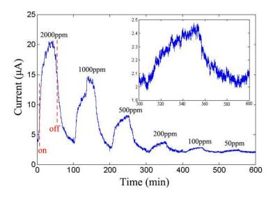
**Figure 6.** Evolution of nanodevice current with respect to the concentration of CO gas at 200 °C (inset is the zoom-in image when the CO concentration is 50 ppm).
