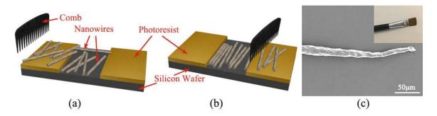
**Figure 1.** Schematic diagram of the combing process. Nanowires array before (**a**) and after combing (**b**). (**c**) A single brush hair of the makeup brush; the inset shows the makeup brush used in practice.
