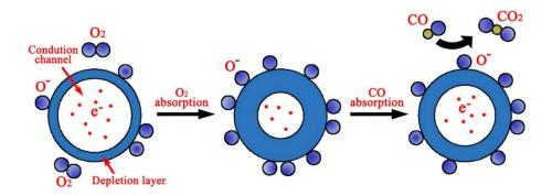
Figure 7. Schematics of ZnO CO sensor sensing mechanism.
