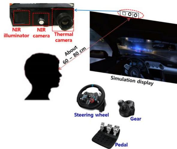
**Figure 2.** Experimental setup for classifying aggressive and smooth driving emotion using multimodal cameras.
