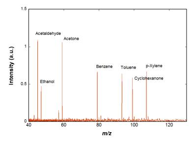
**Figure 4.** Reaction of  $H_3O^+$  ions with a mixture of species diluted in air (acetaldehyde, ethanol, acetone, benzene, cyclohexane, toluene, cyclohexanone, p-xylene, and n-decane) is presented. The  $H_3O^+$  ions do not react significantly with cyclohexane and n-pentane but proton transfer occurs with all the other species, as is observed on the mass spectrum.
