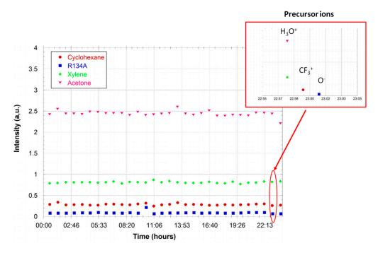
**Figure 9.** Monitoring of the gas injected in an air regeneration unit for a period of one day. Acetone and xylene are monitored using  $H_3O^+$  as the precursor ion. The cyclohexane is monitored using  $CF_3^+$  and  $O^-$  is used for the detection of Freon R134a. The zoom shows the temporal separation of the sequences using the three different precursors.
