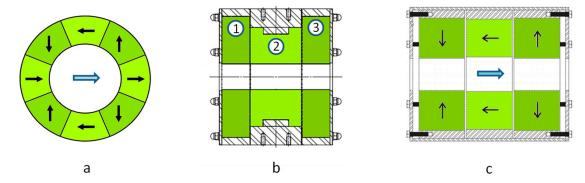
**Figure 3.** Different ways of generating an intense and homogeneous magnetic field using a permanent magnet assembly: (a) Cylindrical structure proposed by Klaus Halbach, here divided into eight segments. (b) Similar structure including three Halbach cylinders (c) Structure producing a field coaxial with the bore. The black arrows in (a,c) show the magnetization direction of the segments, while the blue arrows show the direction of the magnetic field produced in the bore.
