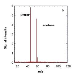
**Figure 5.** Reaction of two different ionic precursors with the same gas mixture, containing four VOCs: acetaldehyde, acetone, butanal, and toluene. (a) With the  $H_3O^+$  ions all four VOCs are protonated. (b) With protonated dimethylether as precursor ions (produced by reacting  $H_3O^+$  ions on a pulse of dimethyl ether), only protonated acetone at m/z 59 is observed, showing a much more specific ionization [30].
