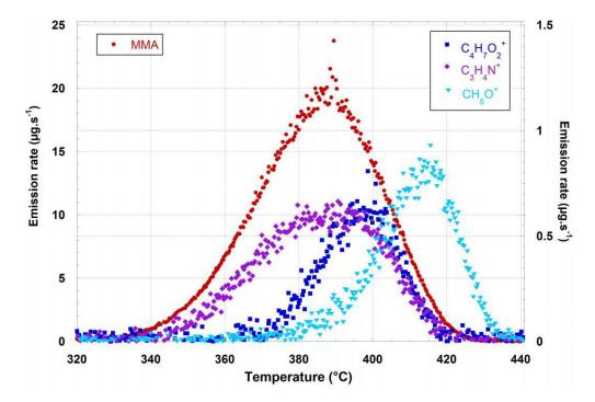
**Figure 8.** Variation of the emission rate of each VOC as a function of oven temperature, for a 3.7 mg PMMA sample heated under a nitrogen flow of 100 mL min<sup>-1</sup>. Left scale = MMA, right scale = emitted VOCs.
