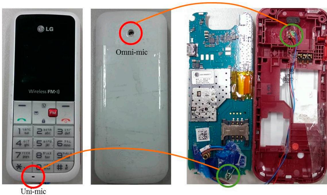
**Figure 3.** Illustration of the dual microphone array in the mobile device.
