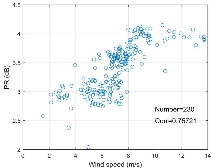
**Figure 11.** The relationship between PR and wind speed of beam 205 data in downwind.
