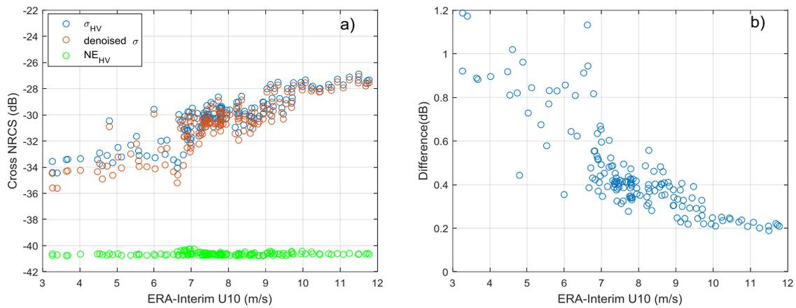
**Figure 5.** (a) The relationship between  $\sigma_{HV}^0$ , denoised  $\sigma_{HV}^0$ , noise floor and wind speed. (b) The difference between  $\sigma_{HV}^0$  and denoised  $\sigma_{HV}^0$ .
