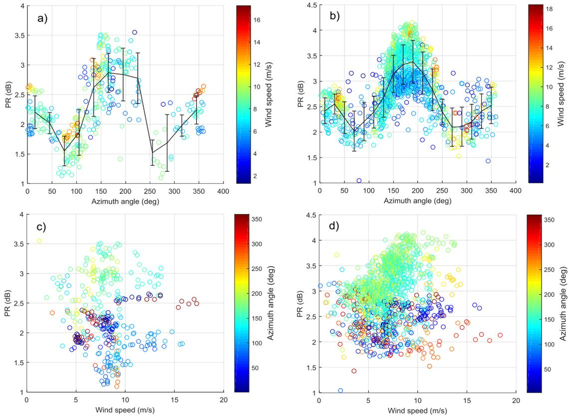
**Figure 10.** (a,b) represent the variation between PR and azimuth angle and different color shows different wind speed. (c,d) show the relationship between PR and wind speed. Different color represents different azimuth. (a,c) are at incidence angle  $39.6^\circ$ . (b,d) are at incidence angle  $41.6^\circ$ .
