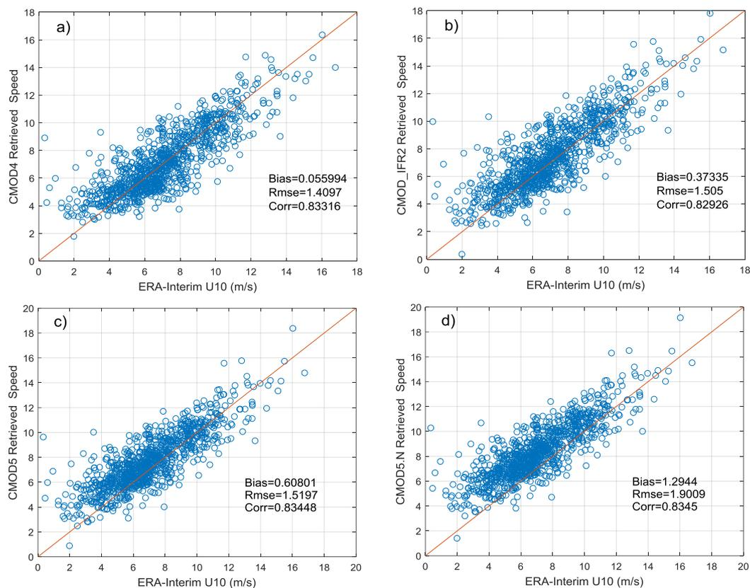
**Figure 13.** Comparison of ERA-Interim U10 with SAR-derived wind speeds which use CMOD4 (a), CMOD\_IFR2 (b), CMOD5 (c) and CMOD5.N (d).
