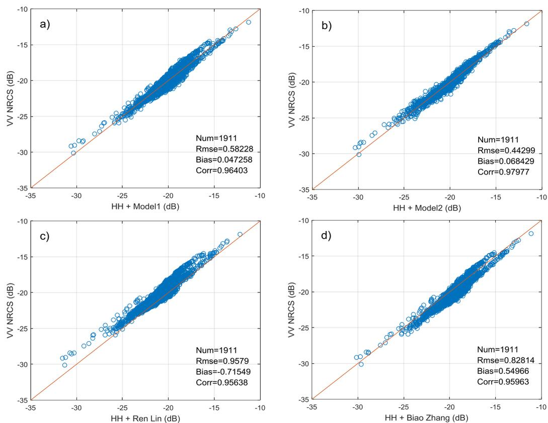
**Figure 14.** Comparison of four different PR models based on testing set where (a) represents PR Model1, (b) represents PR Model2, (c) represents model proposed by Ren and (d) represents model proposed by Zhang.
