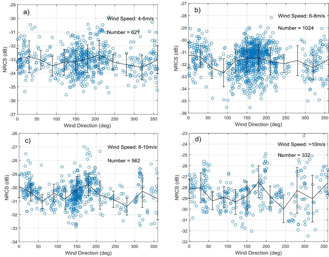
**Figure 7.** Relationship between cross-pol NRCS and azimuth angle at wind speed 4–6 m/s (a), 6–8 m/s (b), 8–10 m/s (c) and >10 m/s (d).
