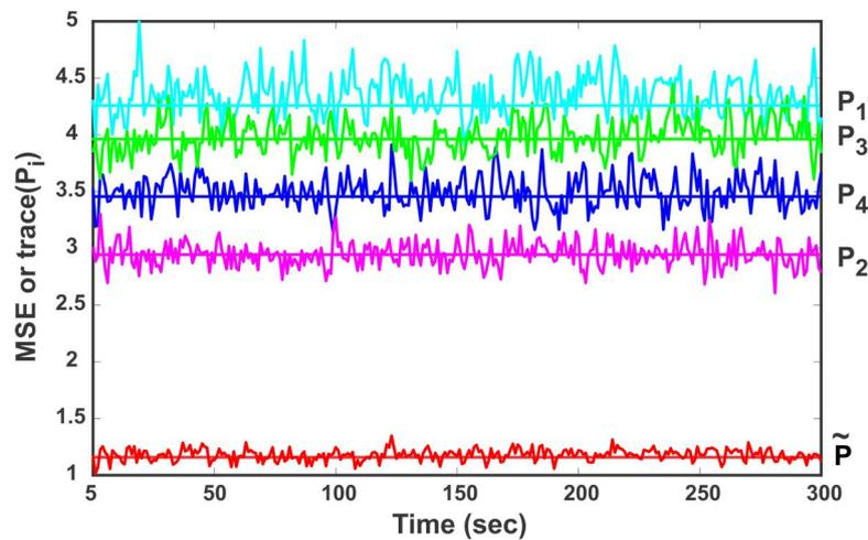
**Figure 8.** The mean square error (MSE) and trace ( $P_i$ ) of local and fused estimates.
