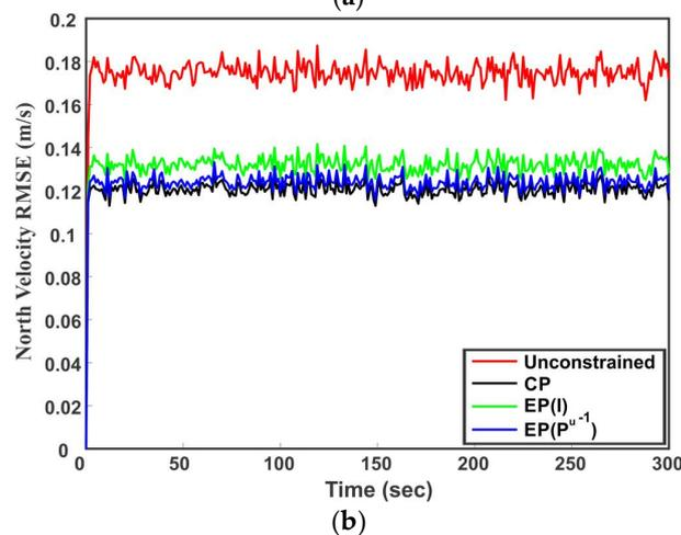
**Figure 10.** Simulation results for the constrained and unconstrained dynamic system. The covariance projection (CP) method is compared with the unconstrained state estimate and estimate projection (EP) method. (a) RMSE of northerly position of vehicle over 1000 runs; (b) RMSE of northerly velocity of vehicle over 1000 runs.
