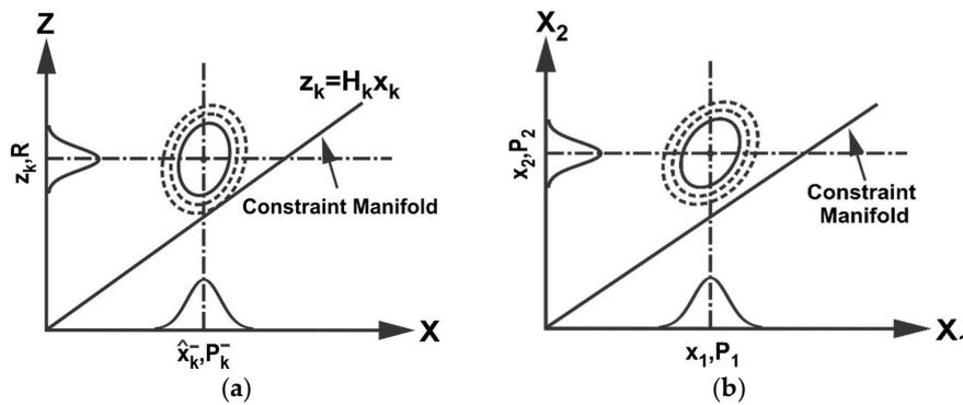
**Figure 1.** (a) Probability of true states and measurements in the extended space around the data from state predictions and sensor measurements and constraint manifold (b) Extended space representation of two data sources with constraint manifold.
